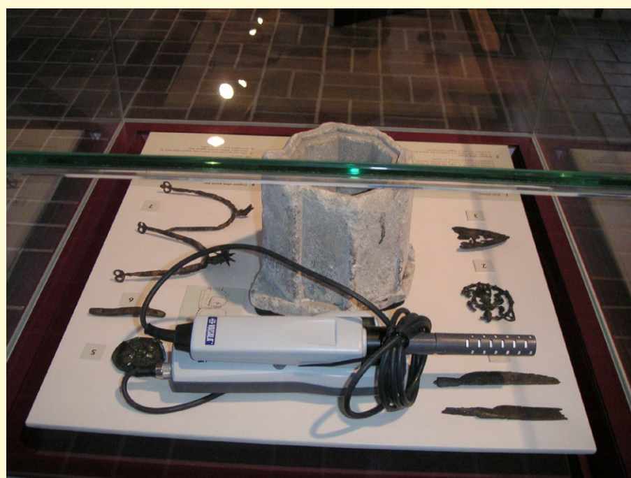
Fig 23. Measuring air exchange rate in a showcase
