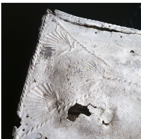
Fig 18. Stable lead corrosion products after Excavation. Lead coffin from St Augustines Abbey
