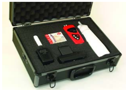
Figure 2. Air exchange measurement equipment case includes gas detector PM3010, Cream whipper and N_2O chargers, external battery and charger. Portable computer also required for analysing data
