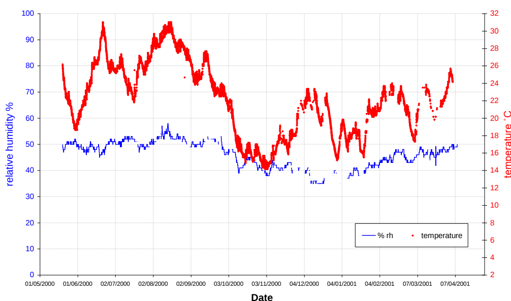
Figure 6.8 Temperature and RH in room adjacent to Blyth Road store room used for the Uley and Stonea material.
