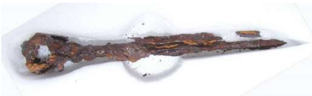
Figure 1.6 Orange akaganeite crystals levering apart Saxon iron pin with eye (Carver 1989).
