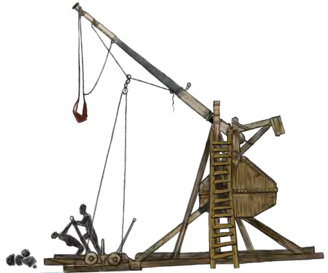
A trebuchet is a giant wooden catapult, with a range of 300 metres, which could throw stone missiles high in the air to smash castle walls.
